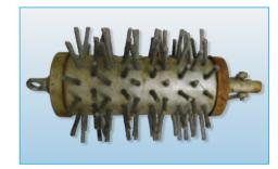
Scraping is a mechanical process in which a device is pushed or pulled through a pipeline to remove built-up deposits on the pipe wall. Because scraping cleans a pipe down to bare metal, this process should always be accompanied by a pipe lining method to prevent accelerated corrosion.
